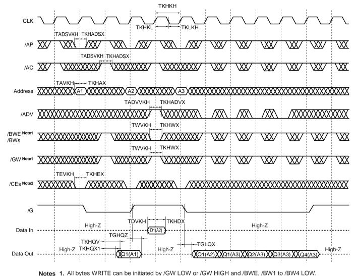
/CEs refers to /CE, CE2 and /CE2. When /CEs is LOW, /CE and /CE2 are LOW and CE2 is HIGH. When /CEs is HIGH, /CE and /CE2 are HIGH and CE2 is LOW.
